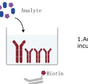
1.Add 100 $\mu\text{L}$  standard or sample to each well, incubate at 37°C for 90 min.
